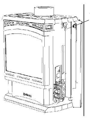
A vent damper is provided to allow fine tuning of the draft. Too little draft will cause flames to be too long with black tips and too much draft will cause flames to be short and blue.
